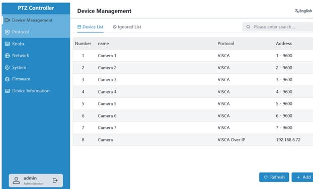
The screenshot displays the PTZ Controller WEB Backstage Management interface. The left sidebar shows navigation options: Device Management (selected), Protocol, Knobs, Network, System, Firmware, and Device Information. The main content area is titled "Device Management" and includes a search bar and tabs for "Device List" and "Ignored List". A table lists 8 devices with columns for Number, name, Protocol, and Address.
