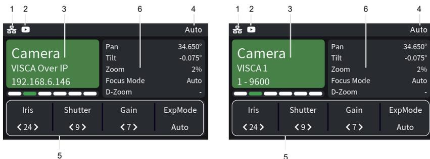
1. Network connection indicator icon“
