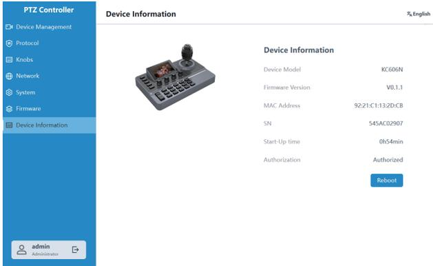
The screenshot shows the PTZ Controller web interface. On the left is a blue sidebar with a menu: Device Management, Protocol, Knobs, Network, System, Firmware, and Device Information (highlighted). At the bottom of the sidebar is a user profile for 'admin Administrator'. The main content area is titled 'Device Information' and features a small image of the controller. To the right of the image is a table of device information:
