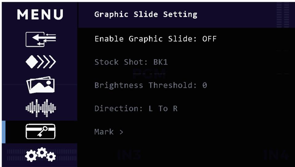
Luminance Threshold: When sliding, the content smaller than the luminance threshold will be deducted, and only the content larger than the luminance threshold will be displayed.
