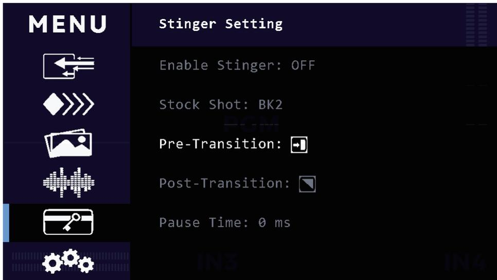
In the process of stinger effects, use the one-way method when using AUTO transition, and use the two-way method when using T-BAR transition.
