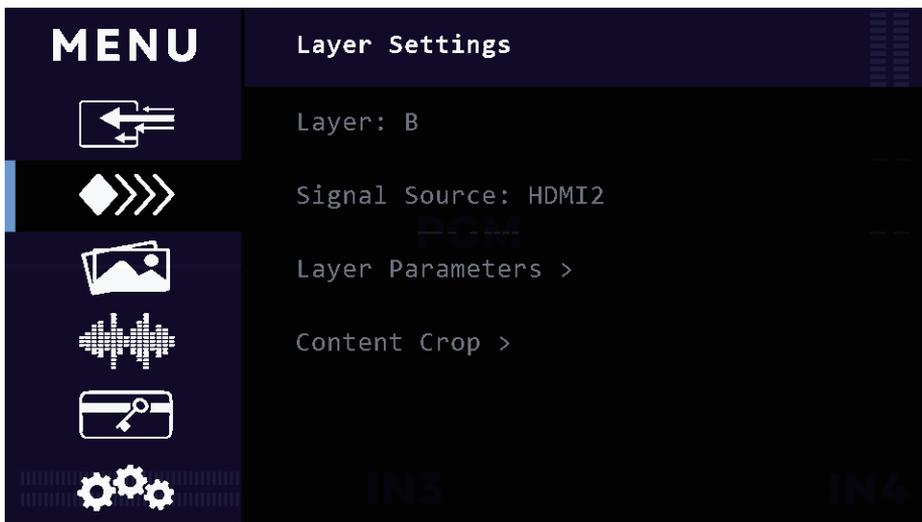
3.2.1 Layer: A layer, B layer or A and B layer can be opened together.
