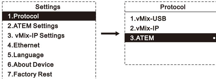
2、ATEM IP setting: After step 1 is completed, short press the CAM1 audio knob to return to the main menu, use the PGM knob to adjust to the second item ATEM Setting, and short press the PGM audio knob to confirm to enter this option. Set the network IP of the ATEM switcher to be connected (please refer to the ATEM device operation manual for the network IP configuration of the ATEM switcher).
