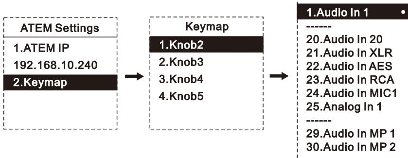
3-2、Introduction of button customization functions: support eight-way buttons PGM9, PGM10, PGM11, PGM12, PVW9, PVW10, PVW11, PVW12 button customization.
